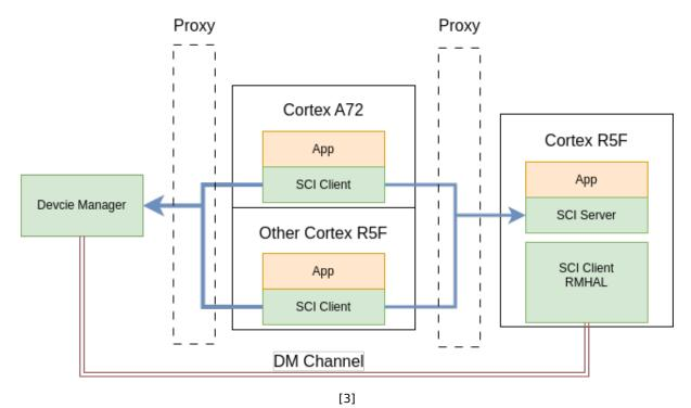
The Cortex-R5F core acts as the SCI server, which means it hosts the TISCI firmware responsible for managing system resources and peripherals while The Cortex-A72 core acts as the SCI client, interacting with the TISCI firmware running on the Cortex-R5F core.
